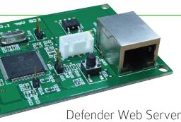
Attach the web server to enable network connectivity, access and control over the network or internet, compatible with Windows and Mac OS
