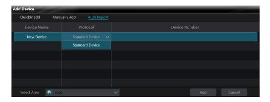
① Input the device name and then select the device protocol.
