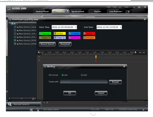
Refer to the interface as shown below. For some devices, you can check "Main Stream" to backup the record by main stream, or by sub stream if you don't check it. The "Main Stream" is enabled by default.
