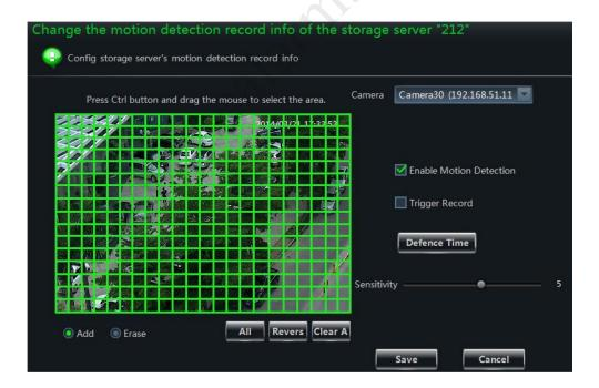
Check "Trigger Record" and then drag the slider to set the sensitivity of the camera. Click "Defence Time" to pop up the "Schedule Setting" window. You can click "System Schedule" button in the window and then select a system schedule in the dropdown menu or set a new schedule for the motion alarm (the settings are similar to that of the local record of device. Please see the schedule setting of the local record of device for details).
