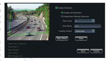
Draw" button to draw the alarm detection area (click around the area where you want to set as the alarm area in the image on the left side to draw a closed area; click "Stop Draw" button if you finish the drawing) and finally click "Save" to save the settings.
