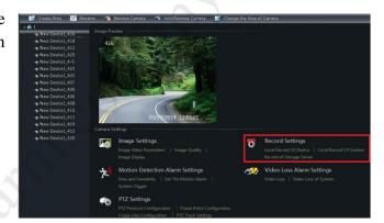
Select a camera and then click *Local Record of Device* to go to the interface as shown on the right.
