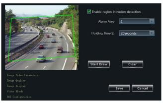
want to set as the alarm area in the image on the left side to draw a closed area; click "Stop Draw" button if you finish the drawing) and finally click "Save" to save the settings.
