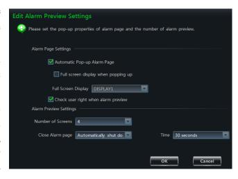
The system will check whether the user which cannot view the live video has the permission to see the alarm preview when an alarm is triggered if the "Check user right when alarm preview" is enabled.
