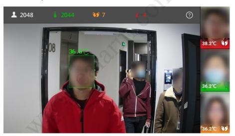
**Figure 8-9 Temperature Screening and Mask Detection**
