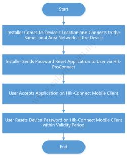
Figure 8-1 Flow Chart of Resetting Device Password
